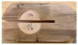
The jig shown was made from pine with a 1¾ inch hole cut using a Forstner bit and a groove cut with a bandsaw. This was a development jig and Roger suggested improvements to prevent splitting could be to make the groove narrower –
