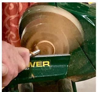
finish the edges whilst the discs are still in the spindle as they become less accessible once in the jig.
