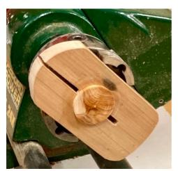
Once the jig is prepared, cut discs that will fit snuggly once the jaws are tightened...the closer the discs are to the 1¾ inch hole, the less pressure and less likely to split the jig. Roger used Yew which is an interestingly figured wood and makes for a good variety of finished pendants.
