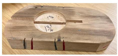
The discs can be shaped as required. The lines shown on the jig are reference points for the edges of the jaw. Once the surface is finished, the edge of the jaw can be moved from the red to the black like, thus moving the centre of the disc, allowing a hole to be drilled off centre.
